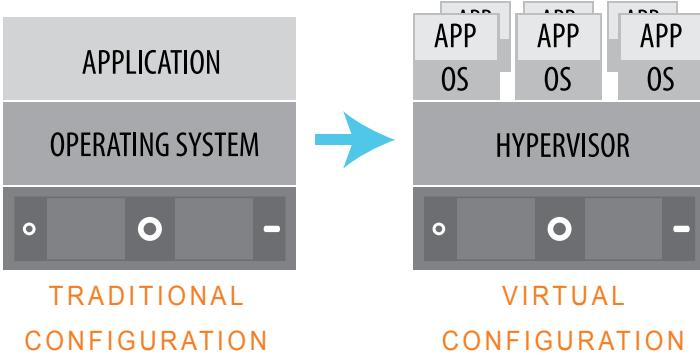
One of the most significant benefits of a virtual environment is the ease of maintenance. Most maintenance activities can be performed live, while the system is running. Not only is it possible to migrate a virtual machine live, it is also possible to replace aging or malfunctioning hardware and balance server load and resources live.
